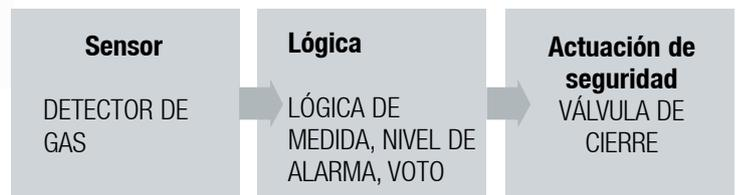
Para SIL 2 PFD (Sensor) + PFD (Resolutor) + PFD (Actuador) <  $1 \times 10^{-2}$
