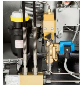
Automatic condensate drain system fitted to a MARINER 320-OX
